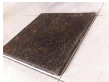
Fig.5 Specimen for thermal property testing of Natural Rubber and Water Hyacinth mixture
